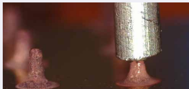
Demonstration of copper pillar three-dimensional (3D) printing with Team Electro3D's new technology. Photo courtesy of Sandia National Laboratories
