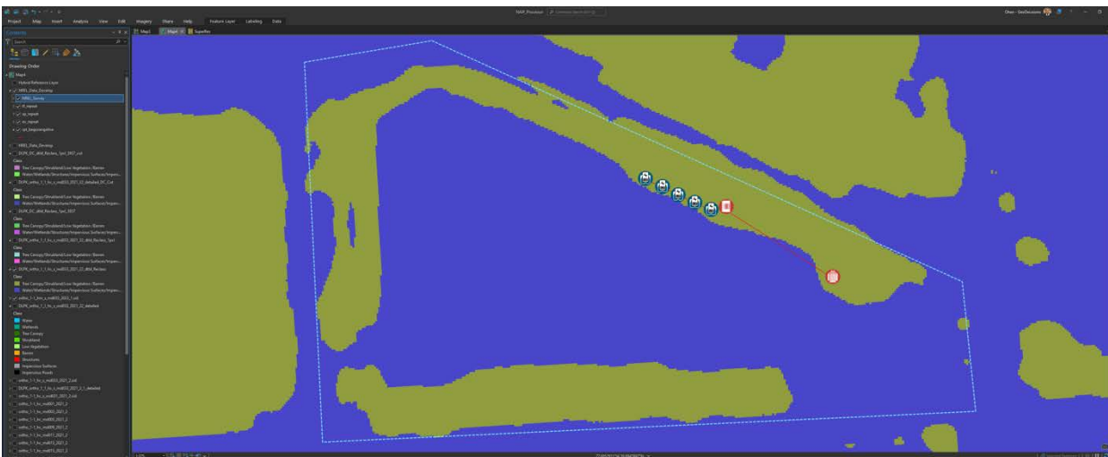
D. Deep pixel classification shows the final classification of permeable and impermeable surfaces at the end.
