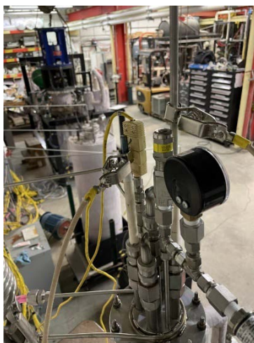
Figure 3.5.5-5. Electrode configuration used for experiment #4.
