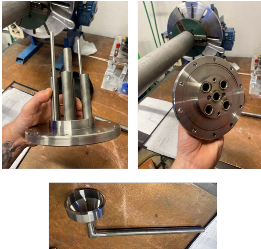
Figure 3.5.3-3. Top of purification vessel (top, left and right) and bottom of reactor vessel (bottom).
