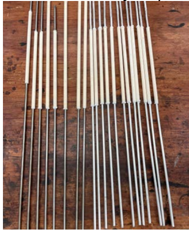
Figure 3.5.3-7. Completed electrode assembly for purification vessel and salt tanks. The castable ceramics were heat cured according to supplier specifications.
