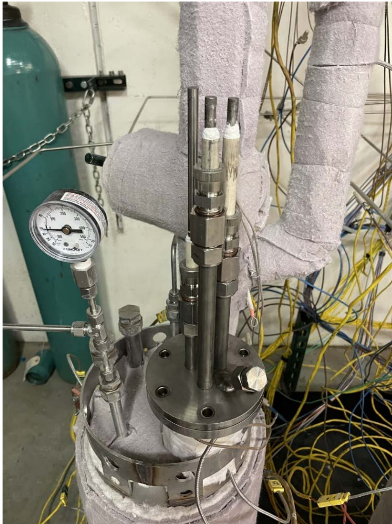
Figure 3.5.4-3. Custom flange on receiving salt vessel with electrode setup for CV.
