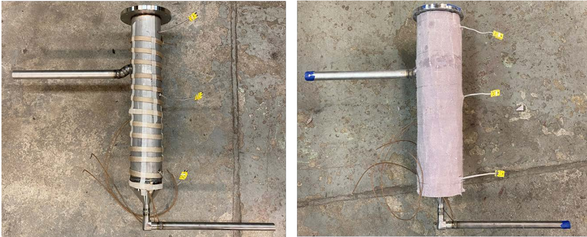
Figure 3.5.3-5. Completed electrode assembly for purification vessel and salt tanks.
