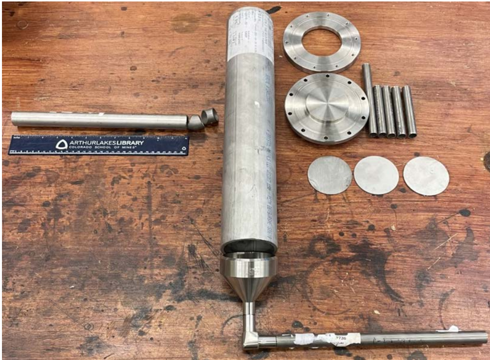
Figure 3.5.3-1. Components of purification reactor as received. The welding of the parts was conducted at the Thermal Hydraulics Laboratory at the University of Wisconsin Madison. Figures 4.1.3.2-2 through 4.1.3.2-4 show the welding process of the parts.
