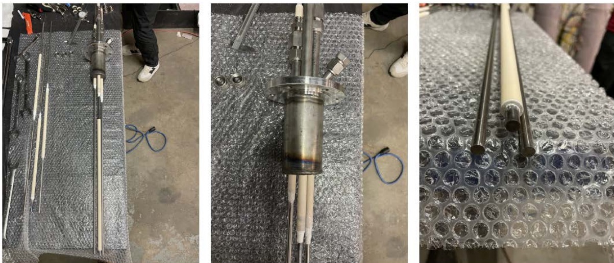
Figure 3.5.4-4. CV electrodes assembly in flange lid of salt vessel.
