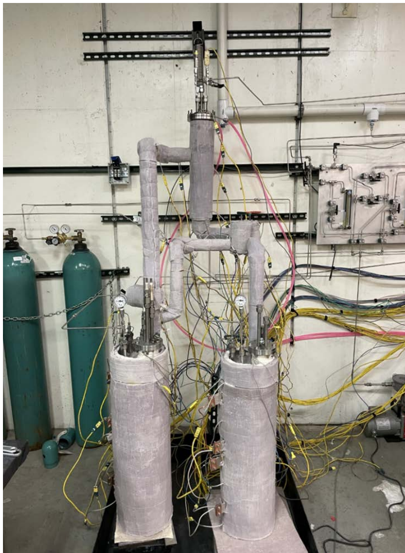
Figure 3.5.1-1. Completed laboratory-scale flow system for evaluation of electrochemical purification method.
