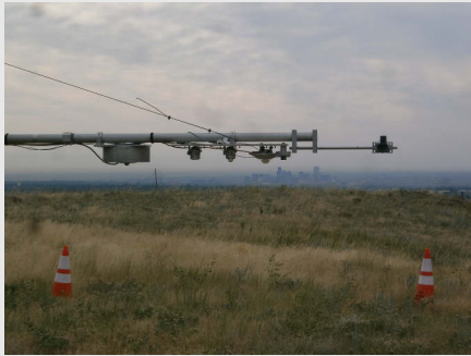
Fig 1. Albedo measurements at NREL's Solar Radiation Research Laboratory.
