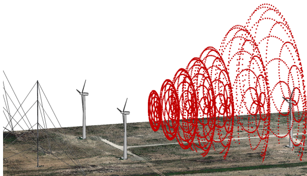
Figure 1: Schematic of SWiFT facility showing the three V27 wind turbines, the meteorological towers located south of the wind turbines, and one of the DTU SpinnerLidar scanning strategies employed for the SWiFT benchmarks (scanning towards the north).
