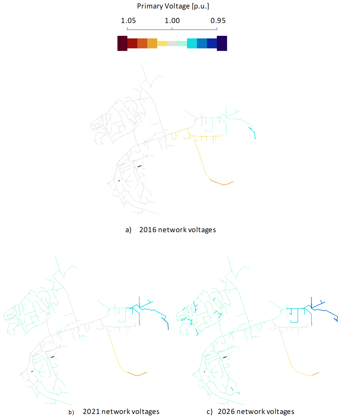
Figure 40. Voltage heat maps for the time step with the lowest network voltage when only existing capacitor banks are operating
